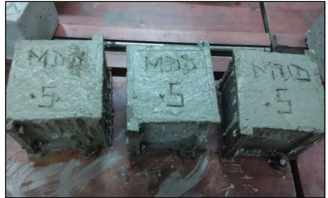
Fig. 4: Concrete cubes casted using nullah water
